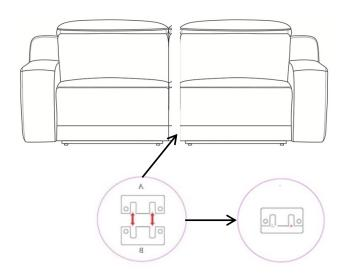
Step8: Plug power parts connection (refer to step 1) into socket at back panel of left and right hand facing recliners, then connect both of them into power source / wall.
