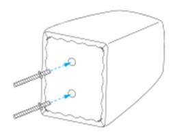
Step4: Carefully tilt the left hand facing recliner forward and lay flat so that you have access to the underside of the chair. Connect the wing to the Left hand facing recliner base by placing the wing with bolts into the pre drilled holes at the rear of the left hand facing recliner arm. Open the zipper pocket at the bottom of the recliner and secure the wing piece to the recliner arm by tightening nuts onto the bolts. Zip up pocket.
